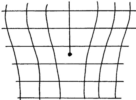
Figure 5. Model of a crystal dislocation.
